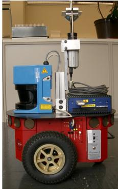
Figure 2: P3DX-platform with omnidirectional camera.
