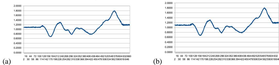
In the building hallway same as above, we measured magnetic field strength with PNI Macromag 3-axis magnetometer. The absolute value in the XY plane is shown in the diagrams above. Since the robot is only moving in XY plane, this value is rotational invariant. We have found the magnetic field anomalies are significant, but remain fairly stable between the first run (Diagram a), and the second run (Diagram b). This means it can assist solving the loop closure problem of SLAM.
