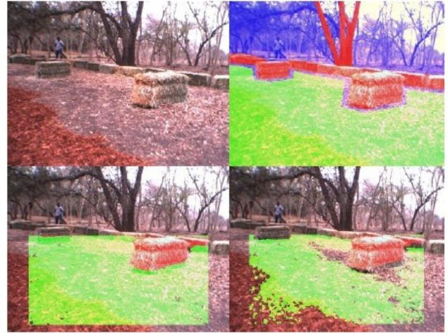
Figure 2. Input Image (Top left), hand labeled ground truth (green: ground plane, red: obstacle, and blue: unknown) (top right), basic auto-labeling output image (bottom left), proposed auto-labeling algorithm output image (bottom right).
