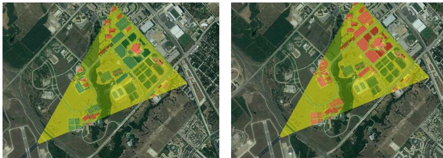
Figure 1. Minimized impact probability maps for an emergency UAV landing at TAMU based on current location and possible trajectories: (a) small UAV during the weekday, (b) small UAV during the weekend.
