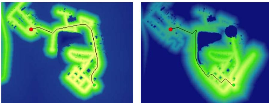
Figure 2. Cost-surface maps for UGV navigation at TAMU based on the current location and intended destination: (a) least-cost path for the UGV, (b) least-cost path adjusted when hazard is marked.
