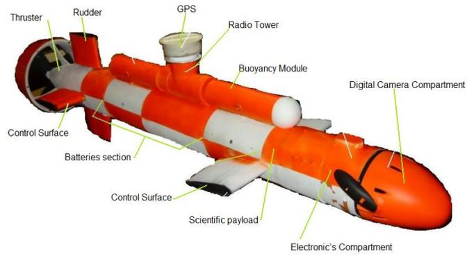
Fig. 1 Mechanical Layout of AUV HIPOPOTAMO
