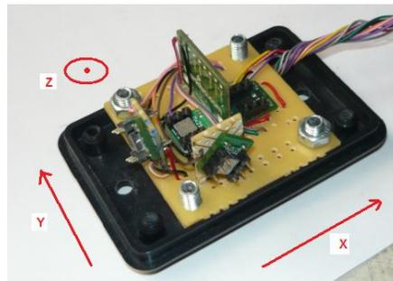
Fig. 2 Inertial Measurement Unit
