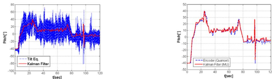
Figure 3. Results for pitch angle. Quanser encoders vs. IMU
