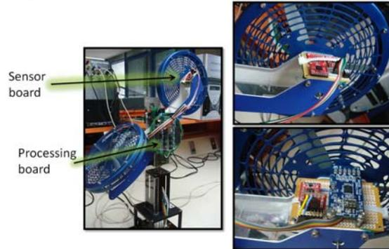
Figure 2. Test set up. Quanser encoders vs. IMU
