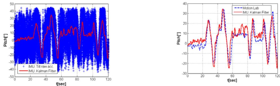
Figure 5. Results for pitch angle. Motion analysis lab vs. IMU
