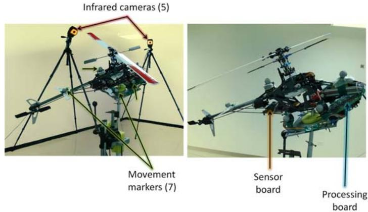
Figure 4. Test set up. Motion analysis lab vs. IMU
