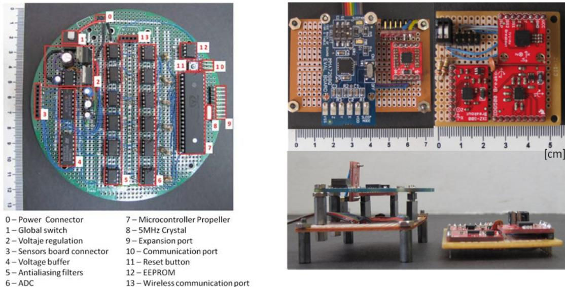
Fig. 1. Prototype of the IMU. Processing board (left), two different sensor boards (right) with gyroscopes of  $30^\circ/\text{sec}$  and  $500^\circ/\text{sec}$
