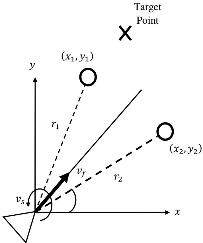
Figure 1 – Diagram illustrating the control problem. The cost function is defined to drive the vehicle toward the target point, while maximizing the distance from the obstacles.
