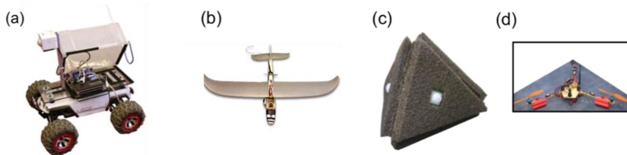
Figure 2. Components used in the SNOOP system were based on COTS technology and modified for the challenge. (a) Wi-fi off-road RC truck (b) RC plane equipped with digital camera (c) SensorMote (d) Tri-copter.
