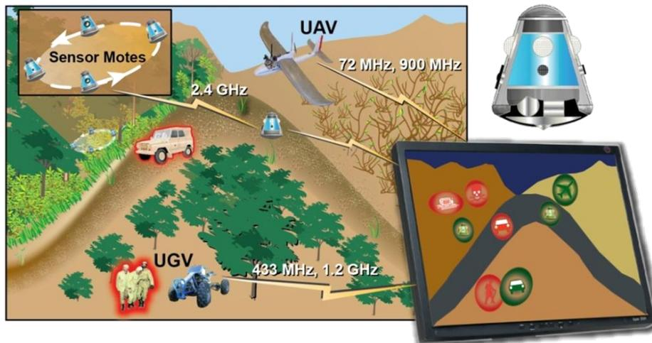
Figure 1. SNOOP system designed with SensorMotes, airplanes, vehicles, and integrated map.
